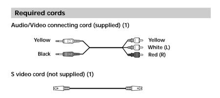
When connecting the cords, be sure to match the color-coded cord to the appropriate jacks on the components: Yellow (video) to Yellow, Red (right) to Red and White (left) to White. Connect the Black jack of the audio/video connecting cord to AUDIO OUT (White) on the player. Be sure to make connections firmly to avoid hum and noise.
